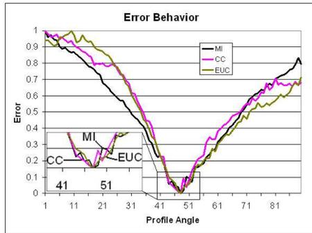
Fig. 5. Comparison of EUC, CC and MI
